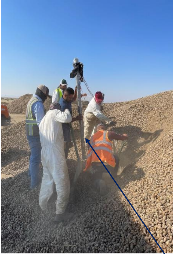
Probes with live video cameras and temperature and relative humidity sensors to Investigate insect infestation and its location characteristics
