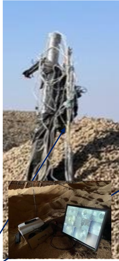
Probes with live video cameras and temperature and relative humidity sensors to Investigate insect infestation and its location characteristics
