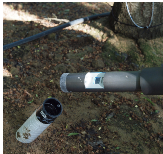
Using a specialized camera, researchers identified the location of the active roots most responsible for nitrogen uptake.
